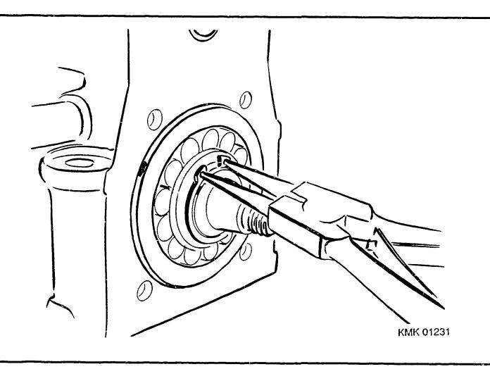
REMOVAL OF CAMSHAFT — CYLINDRICAL—ROLLER BEARING
